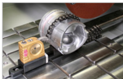
Guide bar with chain clamping vice
